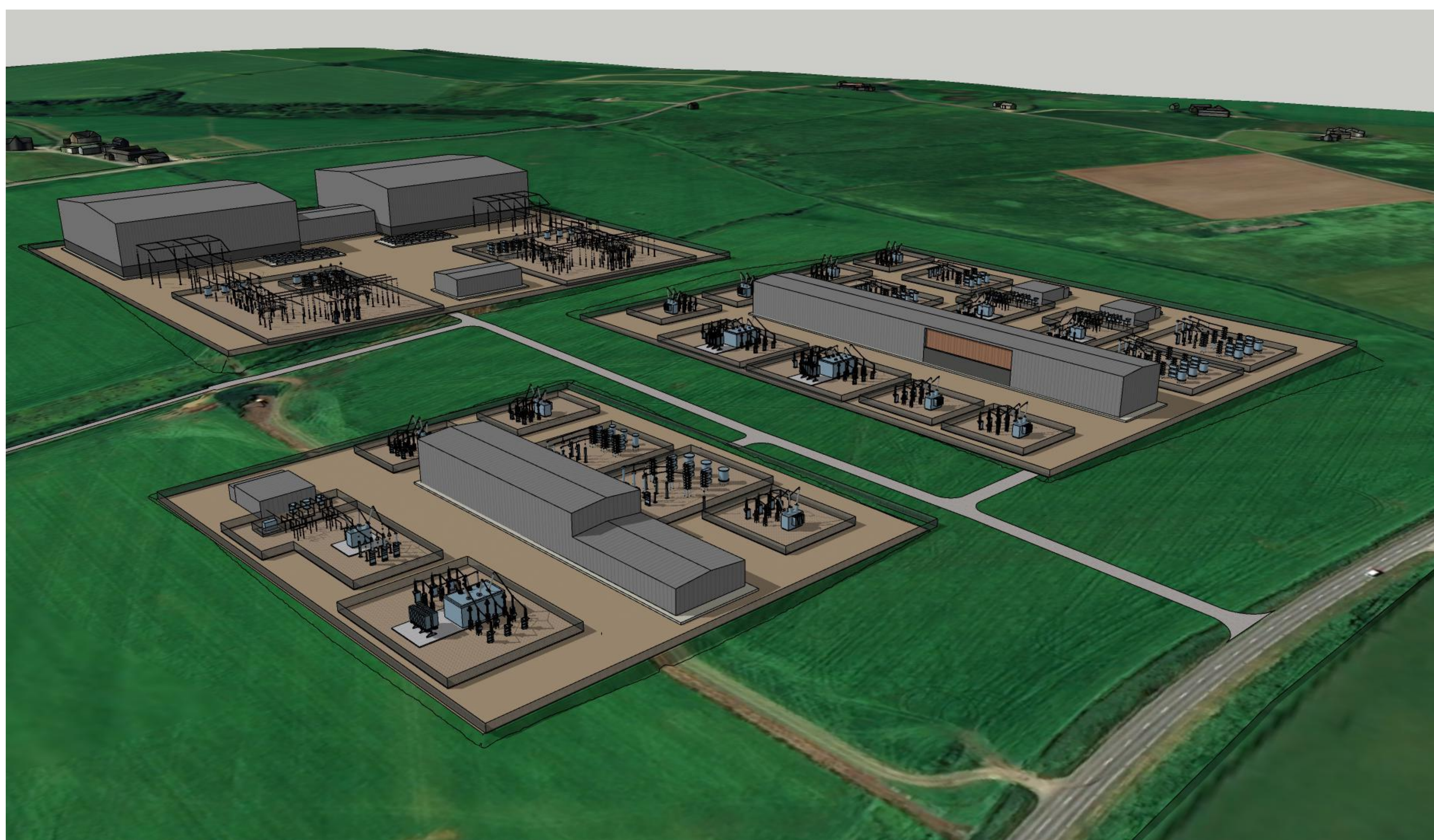
Illustrative conceptual design for a partially enclosed substation site (without visual screening)
